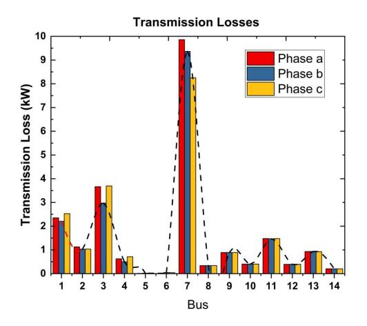
Figure 6: Per Phase Transmission Line Losses for maximum Demand
