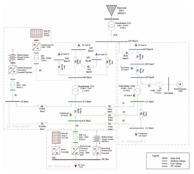
Figure 1: AC - DC Microgrid Architecture
