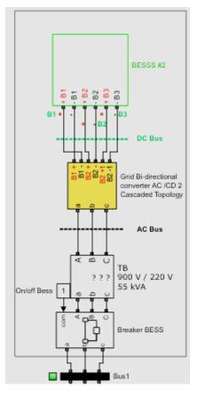
Figure 2: Battery Energy Storage Sub System Connected at Bus 1
