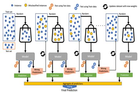
Fig. 2: Internal working of boosting algorithm
